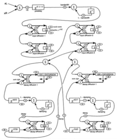
Fig. 1. Simplified plate-class reverberation topology in the style of Griesinger. For output tap structure  $(y_k, y_k)$  see Table 2. Delay-line taps at nodes 24 and 48 are modulating.
