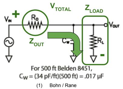
Resistive Voltage Divider: R<sub>L</sub> > 10 \* R<sub>O</sub>
