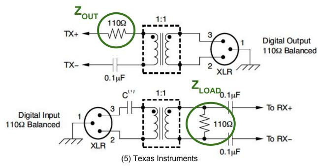
AES/EBU inputs and outputs are designed for a 110-ohm transmission line, so use 110-ohm cable!
