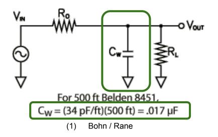
RC Low pass filter  $f_c = 1/(2\pi^*R_o^*C_w)$
