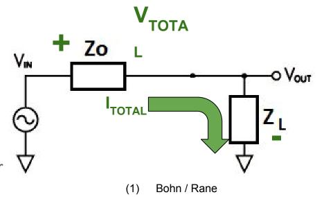
• For fixed max voltage, interface power is determined by input and output impedance
