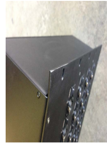
Stage box for snake. Note the bent corner.
