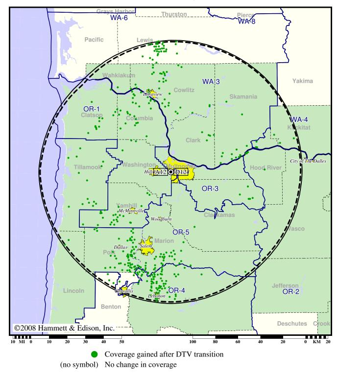
CP (solid): 745 kW ERP at 510 m HAAT vs. Analog (dashed): 1700 kW ERP at 363 m HAAT
