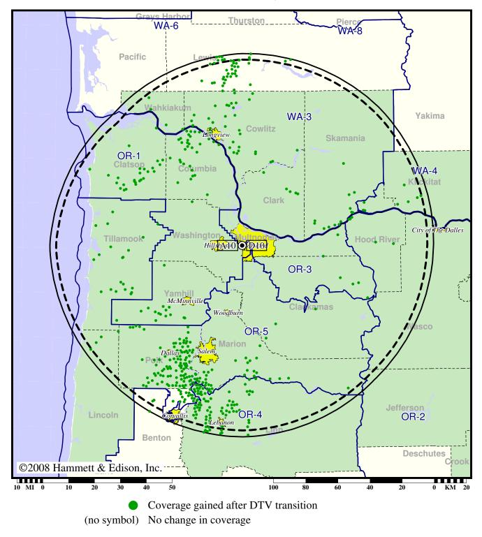
CP (solid): 1000 kW ERP at 513 m HAAT vs. Analog (dashed): 2950 kW ERP at 527 m HAAT
