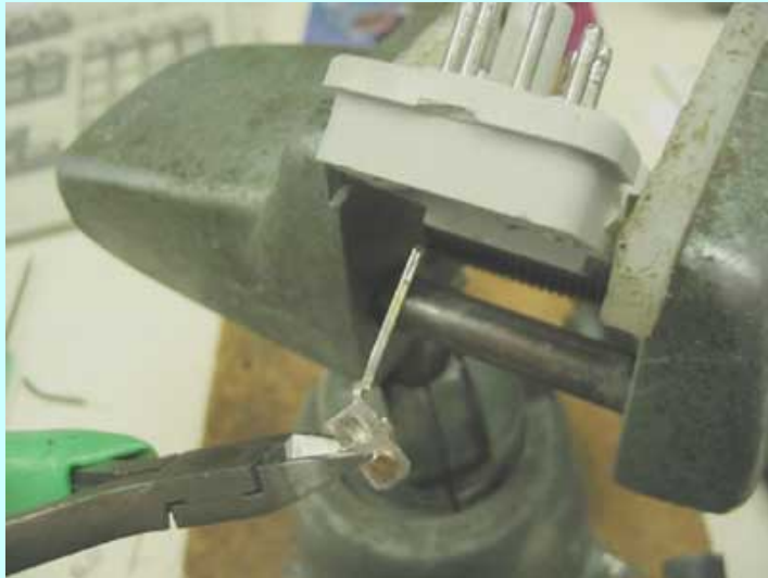
Removing the old relay wires from the octal base.
