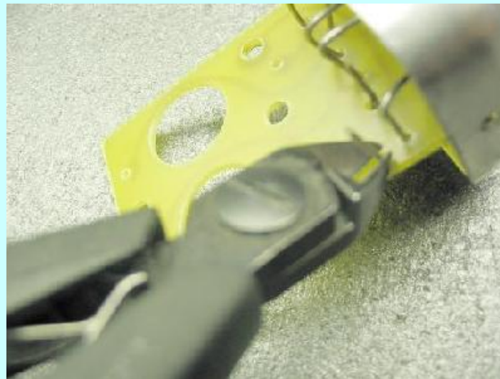
Trim the leads but be careful not to cut the wrong ones! It's very easy to do! Trust me!
