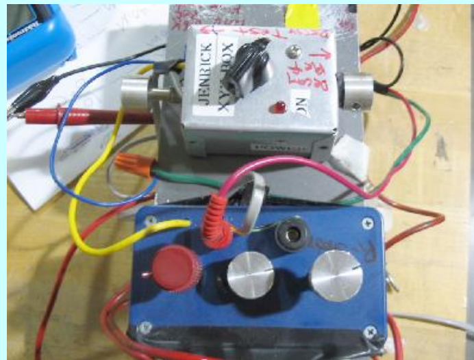
Course, medium and fine adjustments for LED light level.
