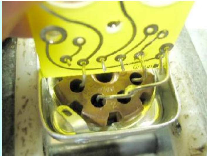
Showing the routing of the wire 1-2 combination.
