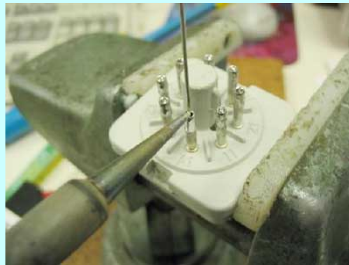
Heat the pin so you can drop the wires in.
