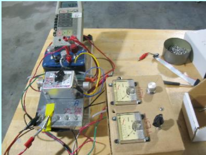
On and Off Resistance jig and decay tester.
