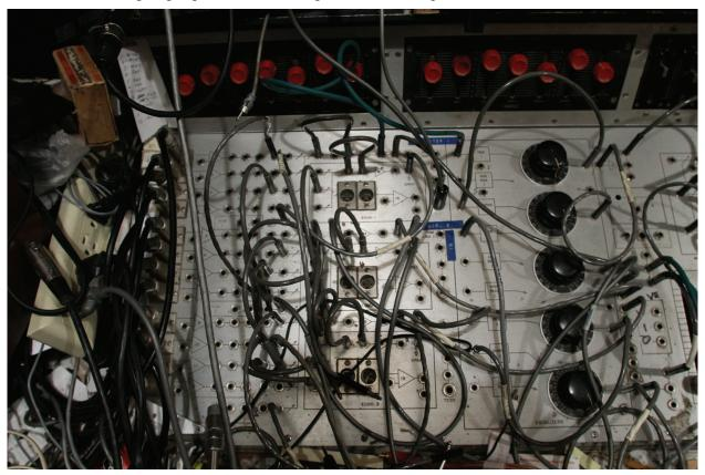
The picture above shows the console configured for use. Perhaps now you can get a feel for how this is used and what is meant by the one-line diagram being the panel of the mixer.
