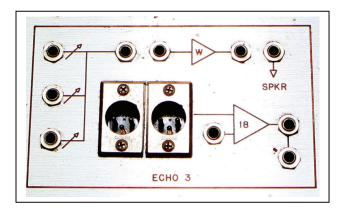
In use, you create the equivalent of a prefader send by multing the signal at the top of a fader, sending it to one of the 3x1 mixers, and then out to the chamber. The chamber returns to an AM-16, which is then patched to the echo return fader input of the 5x1 mixer.
